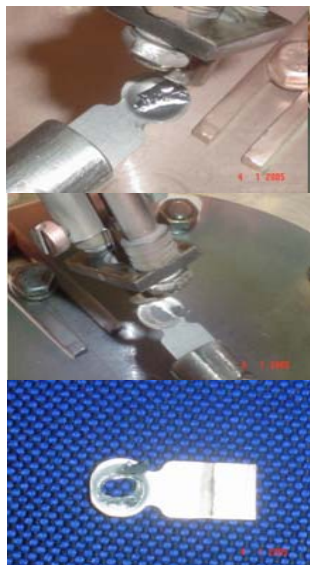
Fig. 3. Wolfram crucibles for deposition of boron. The last photo-image show damaged crucible from tungsten.
