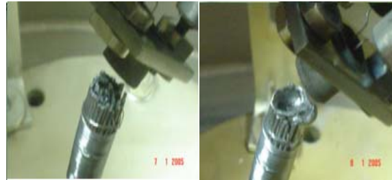
Fig. 5. Wolfram Wires Crucible for deposition of boron.
